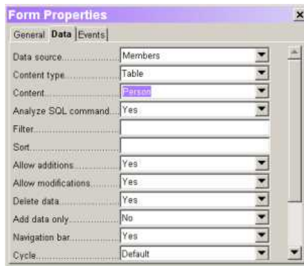
Figure 2. The Data tab of the Form Properties dialogue lets you specify the data source for a form.
